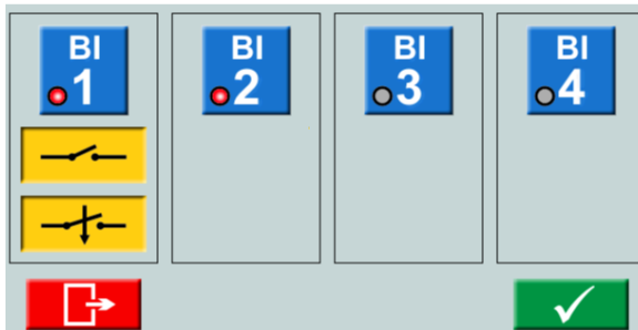
Figure: BI settings for SVERKER 900. Reaction on OPERATE signal
