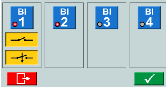
Figure: BI settings for SVERKER 900. Reaction on operate (trip) signal
